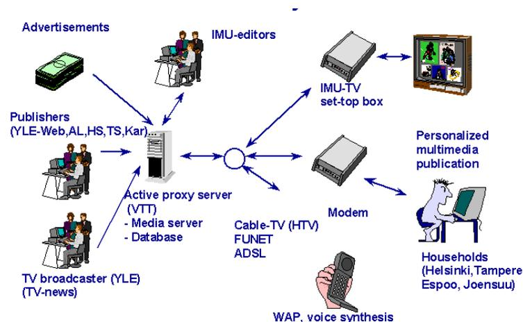
Figure 2. The trial set-up, where the active proxy server processes the content from the media houses. The IMU editors control the machine-made choices and produce own news packages. The publication is used on different terminals.
